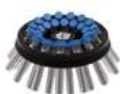
Cabezal angular | GLK008 15mLx30 5000rpm/4100xg Precio 899,00
